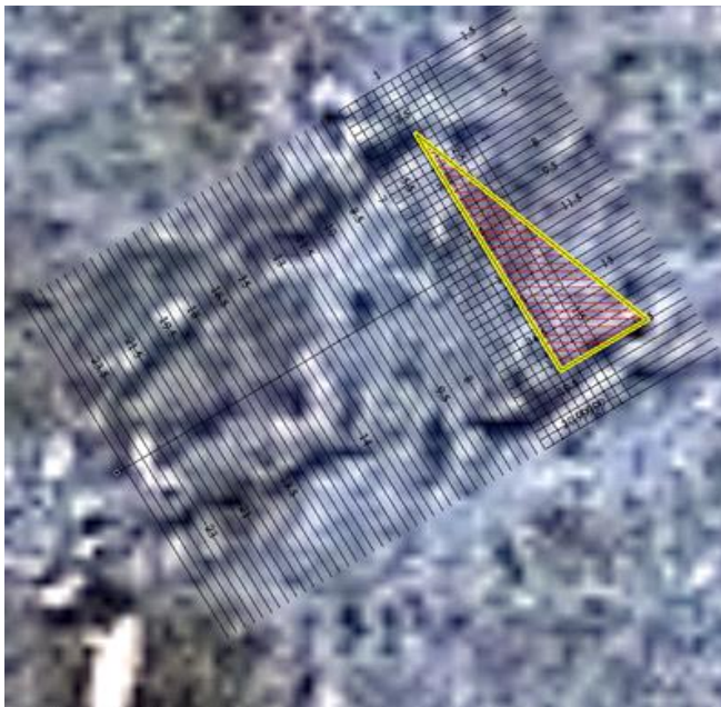
Fig. 5. Satellite photo of ground traces from 11-th of April 2010 (bought from GeoEye). The traces agree with the calculated rotation of the plane and the wing shortened by several meters more than explained by only losing the wing tip.
